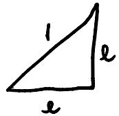
$$\begin{aligned} l^2 + l^2 &= 1 \\ 2l^2 &= 1 \\ l^2 &= \frac{1}{2} \\ l &= \frac{1}{\sqrt{2}} \end{aligned}$$
